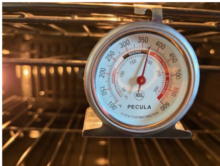
Stand-Alone Oven Temperature Test at 350°F - Reading 370°F
