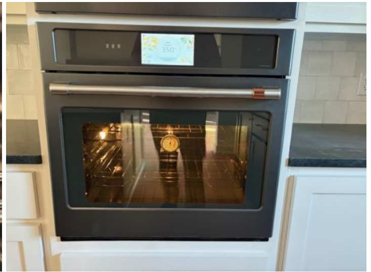
Stand-Alone Oven Temperature Test at 350°F
